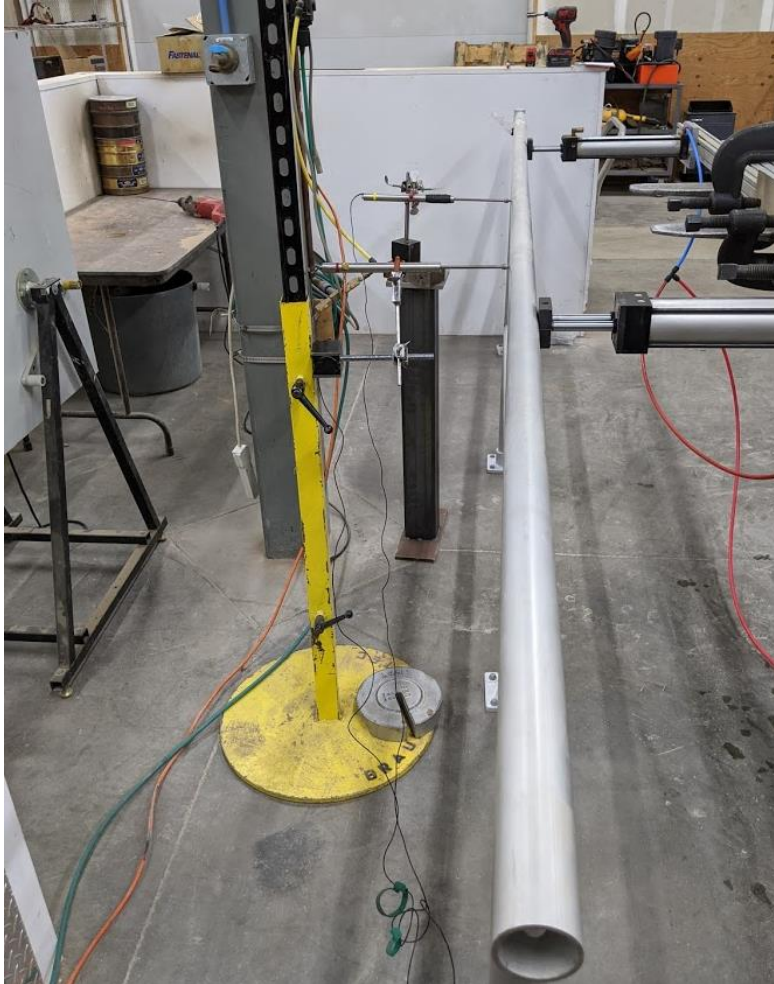
Figure 4: Test Setup – Quarter Point Load
