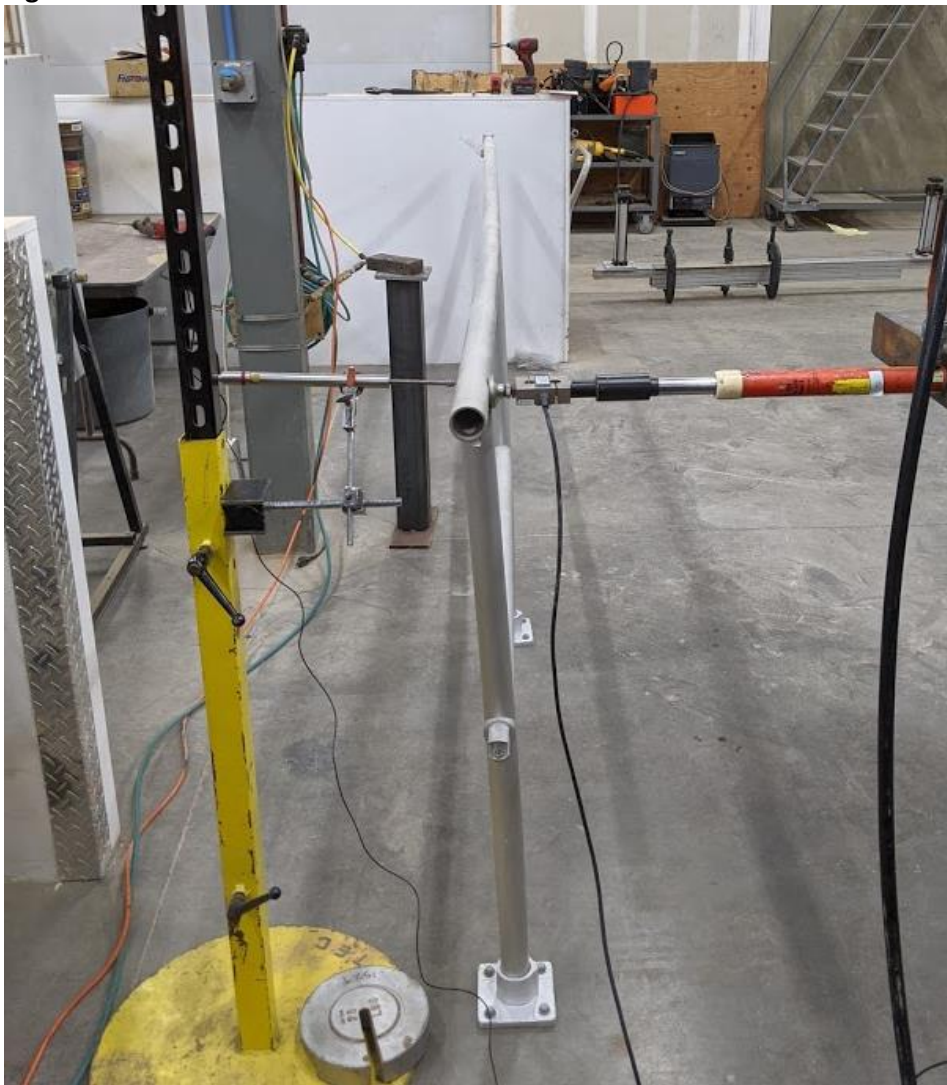
Figure 5: End Post at 200 lbf
