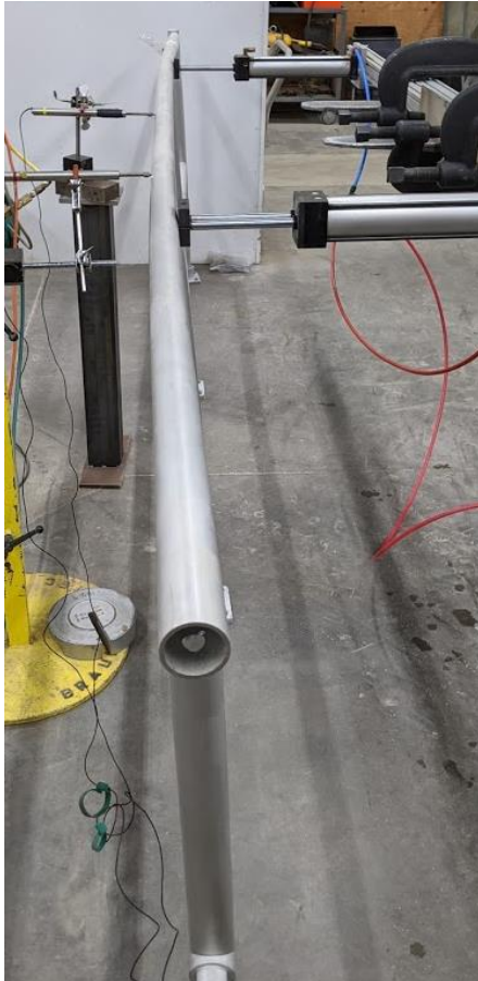
Figure 6: ¼ point load at 608 lbf
